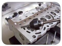
1.2 Insert the REAMER PACKAGE in an Air Drill. The proper drill should exceed 1000 rpm's, UNDER LOAD. Next, choose the appropriate 60° SEAT COLLAR for your application.
