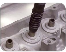
2.3 The Auto-Driver will install the Bronze-Liner "FLUSH", and any excess will be protruding out of the other side. CAUTION: Distortion will occur on the Bronze-Liner if too much power is used, making sizing difficult.
