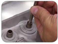
3.2 Hold the tip of the BALL DRIVER with your finger and thumb, with slight down pressure, start driving the Ball. Once the driver tip is inside, relocate your hand underneath to catch the Sizing Ball.
