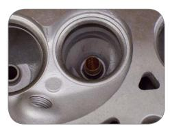
**3.3** Note the excess material protruding. This will be trimmed off in the next operation.
