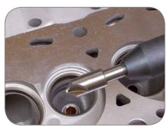
4.3 If a "burr" is created during this operation, it can be removed with the CHAMFER TOOL the has been installed in a "T" handle.
