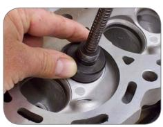
1.3 Insert the Reamer Pilot into the valve guide to be bored, and hold the 60° Seat Collar down on the valve seat. Ream time should be about 5 seconds.
