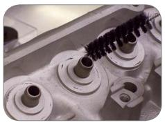
2.1 Once all the guides are bored oversize, turn the cylinder head over so the "spring side" is up. WET BRUSH each bored guide with a nylon brush and lube, such as WD-40.
