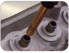
2.2 Insert the Auto-Driver in a "Short Stroke" Pneumatic Hammer (more than 3,000 blows per minute), set the regulator at about half, and install the Bronze-Liner. Installation time should be about 3 to 5 seconds.
