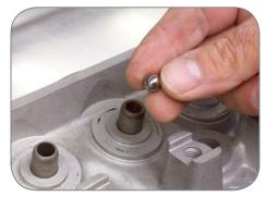
3.1 Select a Carbide Sizing Ball .001" larger than the desired finished size, as the Bronze will spring back slightly after Ball Sizing.
