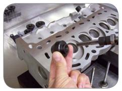
1.1 The first operation is to install the parts from the Reamer Kit onto the Boring Reamer. Install the BUSHING, then the SPRING, and finally the RETAINER. You now have a Reamer Package.
