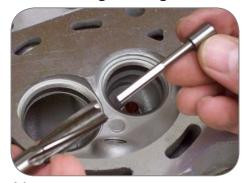
4.1 Insert the appropriate PILOT into the TRIMMING TOOL. Install the Trimming Tool into a 500 rpm drill.
